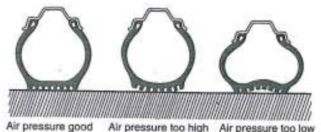
Relationship between tire air pressure and deformation
